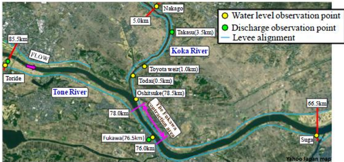
Figure 1 Study area and location of observation points in and around the Fukawa contraction area in the Lower Tone River.
