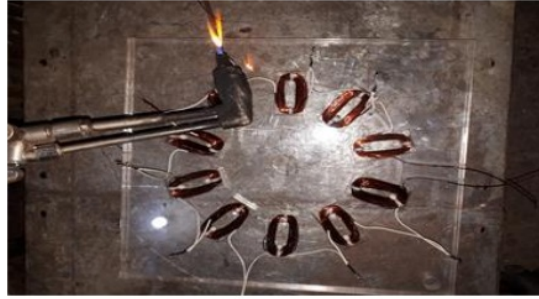
Fig. 11 The winding to the stator installed permanently.
