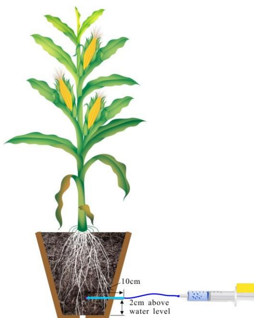
Figure S1.3. An example of a soil water sampler in a 7 L pot
