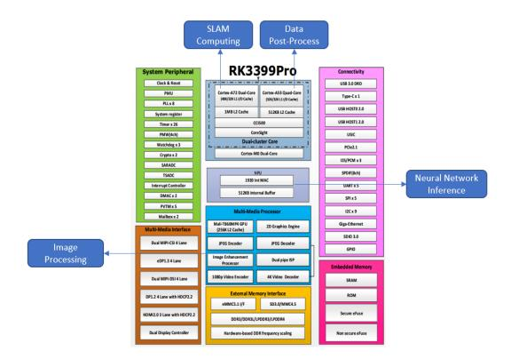
Figure 4-2 RK3399PRO Soc Architecture
