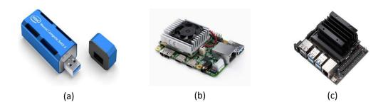
Figure 1-5 Different Edge Computing Platform (a) Intel's Neural Compute Stick (b) Google's Edge TPU Platform (c) Nvidia's Jetson Nano
