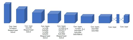
Figure 3-5 Neural Network Structure of YOLO
