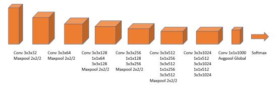
Figure 3-6 Neural Network Structure of YOLOV2
