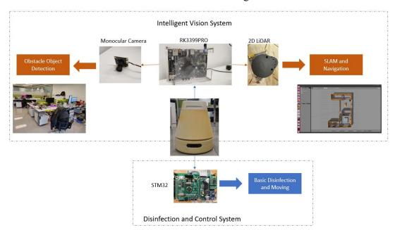
Figure 5-4 Disinfection Robot with Intelligent Vision System
