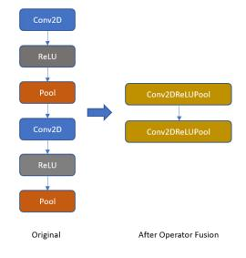
Figure 4-22 Operator Fusion of Pooling
