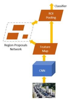
Figure 3-2 Neural Network Structure of Faster-RCNN
