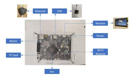
Figure 4-3 Development Board Connection Diagram
