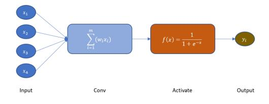
Figure 4-12 Activation Function Process
