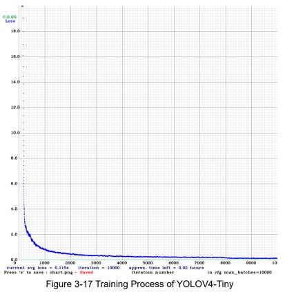
(The Loss function is more stable than YOLOV3 and YOLOV4 and has less average loss)
