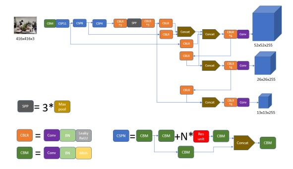
Figure 3-12 Neural Network Structure of YOLOV4
