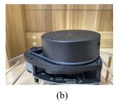
Figure 2-1 Sensors of Vision System (a)Monocular camera (b)2D LiDAR
