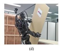
Figure 1-1 Application of Robots (a) Proscenic's sweeper robot (b) iRobot's sweeper robot (c) Xiaomi's CyberDog (d) AIST's HRP-5P
