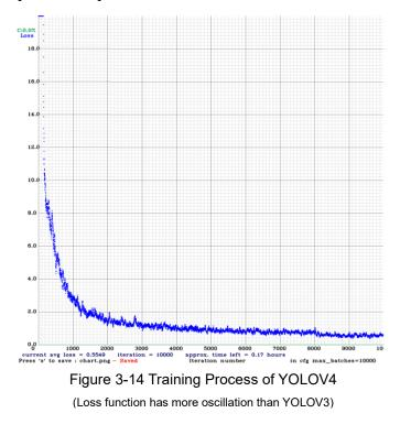
Similarly, on the mobile robot platform in this thesis, the YOLOV4 neural network is selected to train on the MS coco dataset with 80 target classes and own dataset. The training process of YOLOV4 network is shown in Figure 3-14 and the inference results of YOLOV4 network on high-performance server is shown in Figure 3-15.
