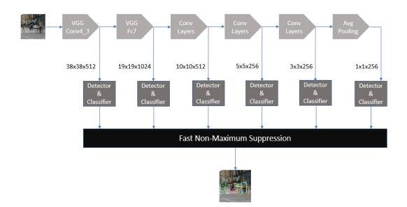
Figure 3-3 Neural Network Structure of SSD
