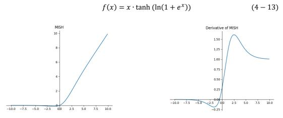
Figure 4-17 Mish Function Curve
