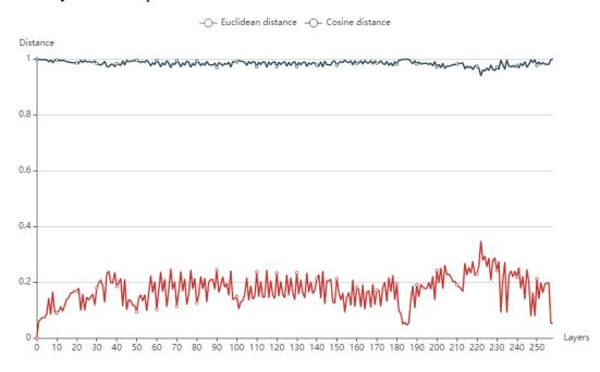
Figure 4-7 Accuracy Analysis of Asymmetric Affine Quantization
