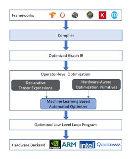
Figure 4-4 Compilation and Optimization Process of TVM
