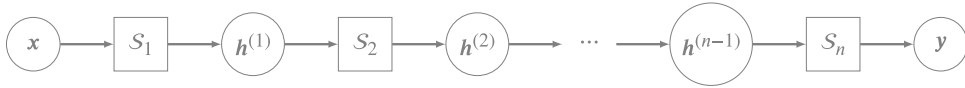
Fig. A.1. Multilayer perceptron: S_1, \dots, S_n denote single layer perceptrons, h^{(1)}, \dots, h^{(n-1)} denote hidden layers, and circles are used to denote input and/or output vectors.
