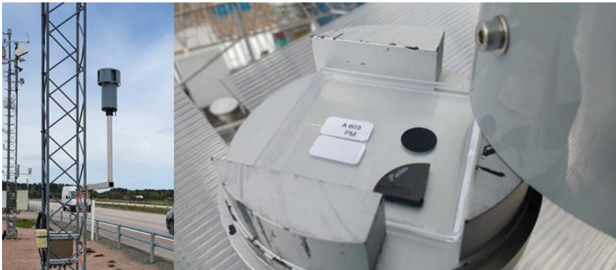
Figure 12. Sigma 2 sampler at Testsite E18. Photo: Mats Gustafsson, VTI and David Jaramillo, Particle Vision.
