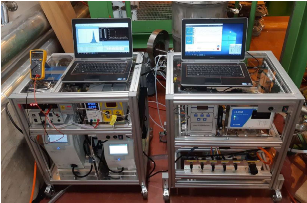
Figure 10 – Modular SID alkali measurement system, as setup on the D-CFB pilot
