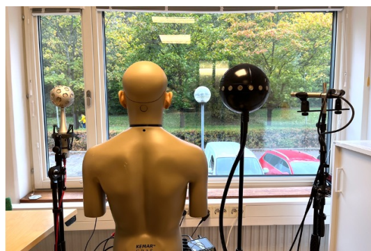
Figure 1: Indoor road traffic noise measurement setup.
