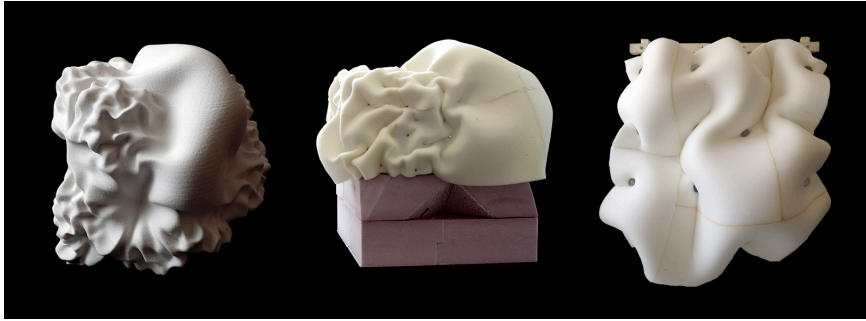
Figure 3.12. Erratic , feedback loops between simulation and material tests: 1:25 scale model created with physics simulation (left), 1:5 scale analogue model (middle), and 1:1 scale mock-up (right).
