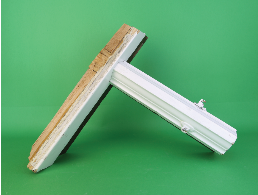
Figure 3.13. Completions , photogrammetry scanning process to obtain a closed mesh model. Greenscreen photograph of salvaged window frame.
