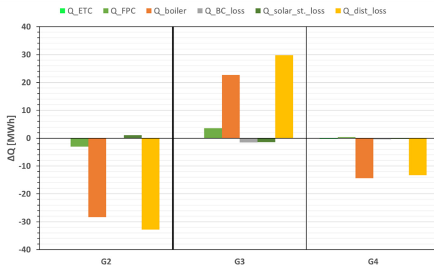
Figure 9. Energy balance difference—Relative changes in lost and supplied energy compared to the reference variant (G1) for the variants of the GRUDIS concept. The bold line indicates a change in pipe manufacturer; G1 and G2 employ M2, while G3 and G4 employ M1 and M3, respectively—see Table 7 for overview.
