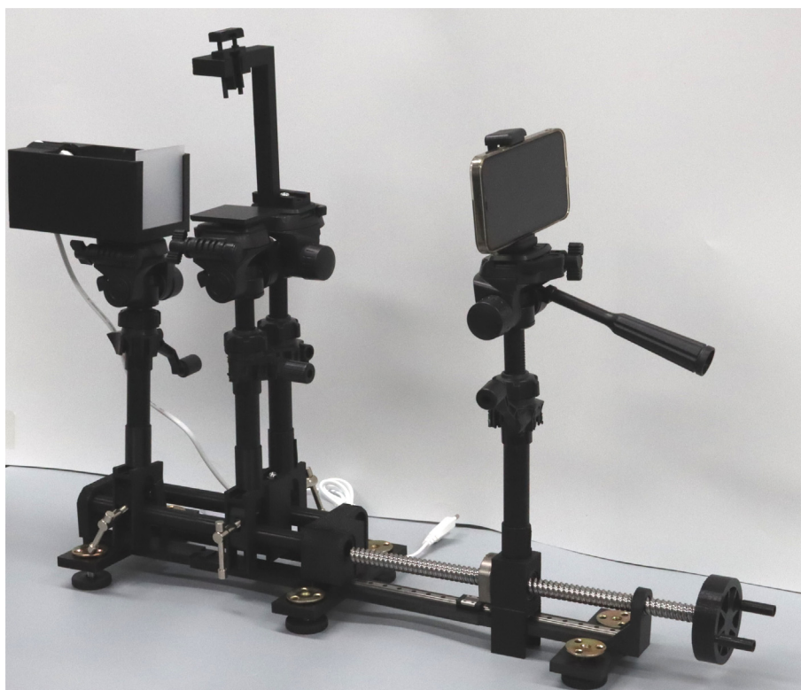
Fig. 9. Photo of the assembled contact angle analyzer showing the light box module, sample plate module, volume metering module and camera holder module (from left to right).
