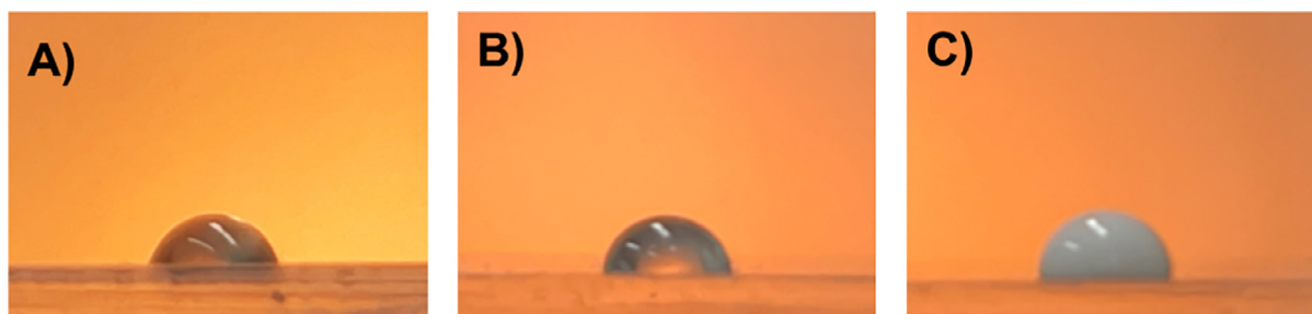
Fig. 14. Beverage drop in volume of 5 \mu L on PDMS A) Lipton Iced Tea, B) Gatorade and C) milk.
