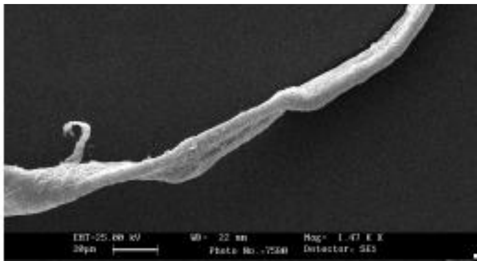
Fig 11. Typical tape structure of a cotton fiber coming from the TS.
