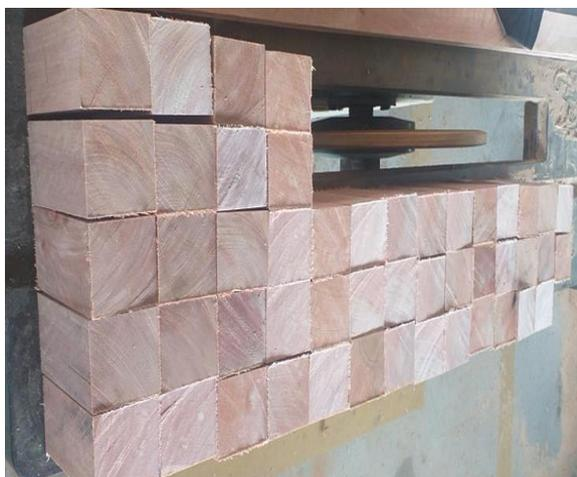
**Figura 31.** Secado al aire de probetas
