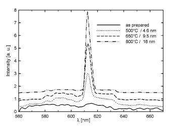
Fig. 3 Luminescence spectra of n-Y<sub>2</sub>O<sub>3</sub>:Eu<sub>2</sub>O<sub>3</sub>(11 mol%) in dispersion upon excitation with wavelength  $\lambda_{ex}=234$  nm in different states of annealing. The plots are mutually shifted in vertical direction. The crystallite size is deduced from XRD line broadening (Scherrer)
