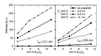
**Fig. 5** Variation of photoluminescence yield in  $Y_2O_3$ : $Eu_2O_3$  with annealing treatment and  $Eu_2O_3$  content for regions of host lattice ( $\lambda_{ex}=211$  nm) and charge transfer excitation ( $\lambda_{ex}=234$  nm)
