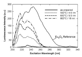
**Fig. 4** Excitation spectra for the luminescence at  $\lambda_{em}=613$  nm  $(5D_0 \rightarrow 7F_2)$  measured on dispersed  $Y_2O_3$ :Eu<sub>2</sub>O<sub>3</sub> particles. Bulk Eu<sub>2</sub>O<sub>3</sub> is shown as a reference
