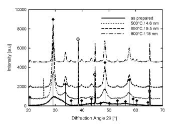
**Fig. 1** X-ray diffraction spectra of  $Y_2O_3$ :Eu $_2O_3$  in different stages of annealing. The symbols  $\spadesuit$  and  $\bigcirc$  denote literature data for  $Y_2O_3$ :Eu $_2O_3$  (5 mol%) and Al (specimen holder) from the PDF-2 database, respectively [10]. No noticeable change is observed for samples with Eu $_2O_3$  addition of 5.6 and 11 mol%
