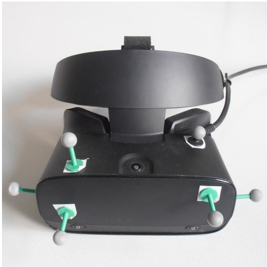
Fig. 3 Oculus Rift S instrumented with reflective markers
