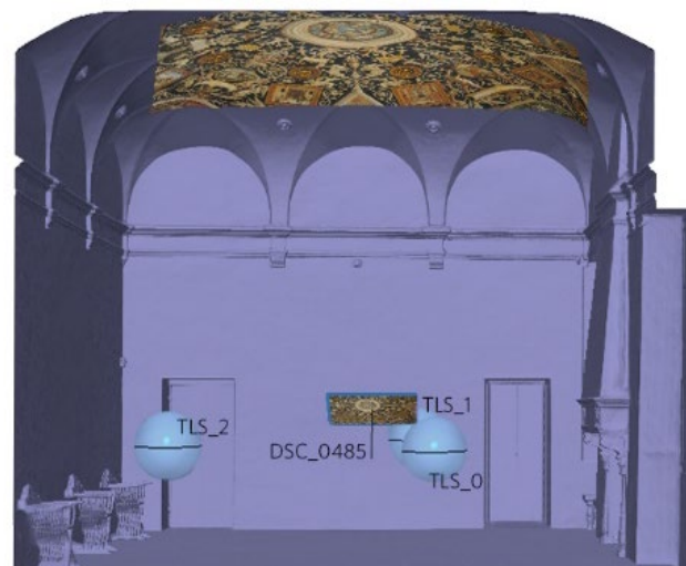
Figure 3. Example of co-registration of a single frame image on the spherical images from TLS (Room 1).
