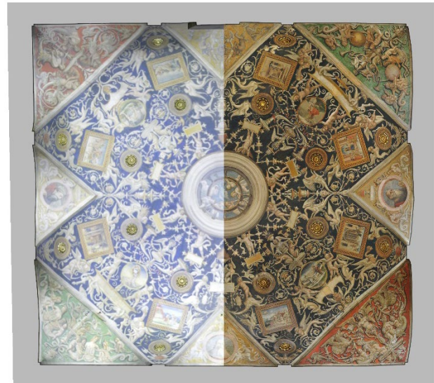
Figure 6. Plan vault of the chamber frescoed by Araldi (on the left: orthophoto computed using the radiometric information provided by the RTC360 camera; on the right: orthophoto computed using the radiometric information provided by the Nikon D3x).
