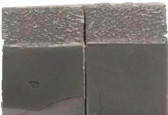
Fig. 4. SLJ exhibiting a cohesive type of fracture.
