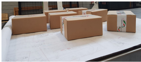
Figure 5: The paper board with the printed configurations of the parcel boxes used as groundtruth.
