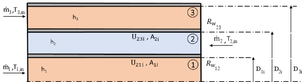
Figure 2. Scheme of the investigated heat exchanger.
