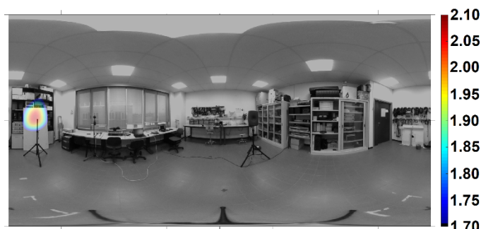
Figure 7: Sharpness map of a pink noise source and a disturbing tone, [acum].
