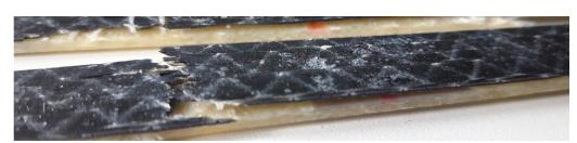
(a) Fiber fracture of Co-SMC (41.0.T20)
