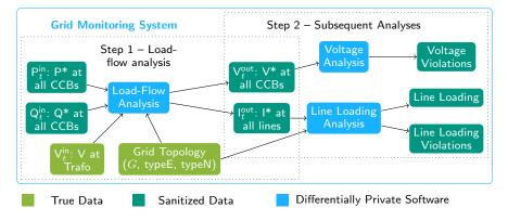
Figure 3: Illustration of the two-step process of grid monitoring.
