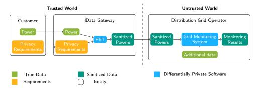
Figure 1: Differentially private grid monitoring. *True* data refers to data that is measured and not sanitized.
