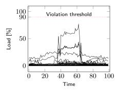
(b) Currents at all lines determined by load-flow analysis.
