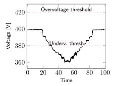
(a) Voltages at all nodes determined by loadflow analysis and the violation es determined by voltage analysis.
