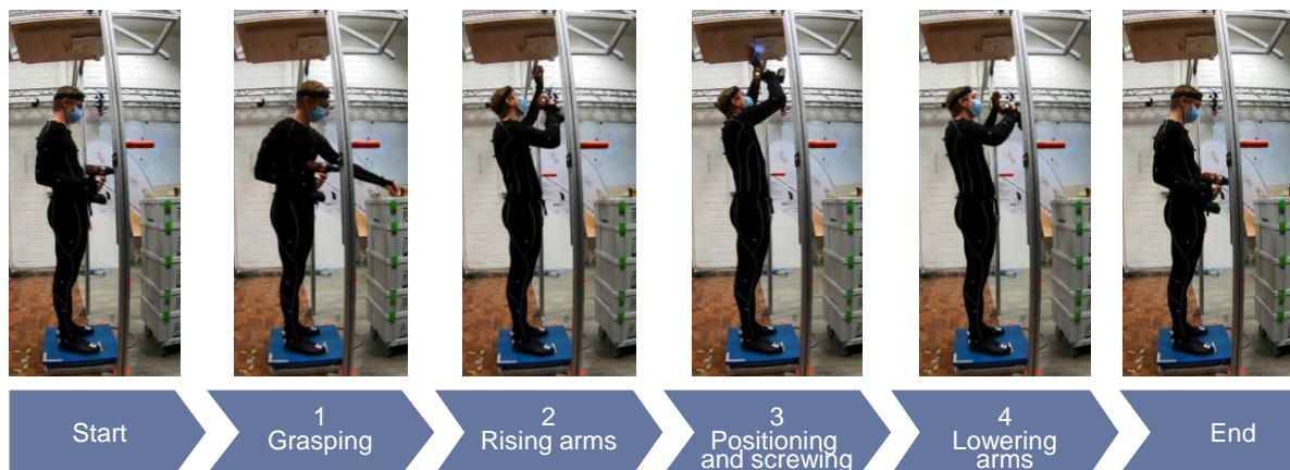
Figure 2. Movement sequence of the selected use case working in and above head height with a power tool
