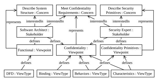
**Figure 5.1.:** Overview on addressed viewpoints and view types including corresponding concerns and stakeholders given as UML object diagram.
