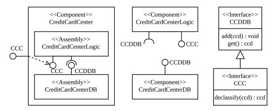
Figure 7.7.: Example illustrating nested assemblies in the CreditCardCenter component.
