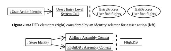
Figure 7.20.: DFD elements (right) considered by an identity selector for a store (left).
