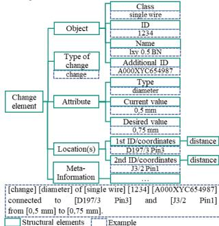
Fig. 3. Newly developed structure for a standardised description of engineering changes with an example depicted in human-readable form
