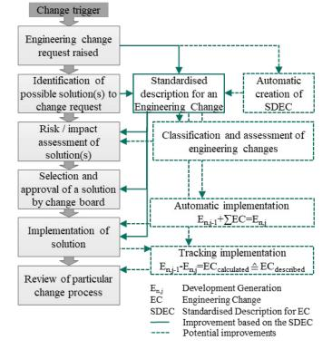
Fig. 8. Potential improvement of the generic engineering change process [6] based on the newly developed standardised engineering change description
