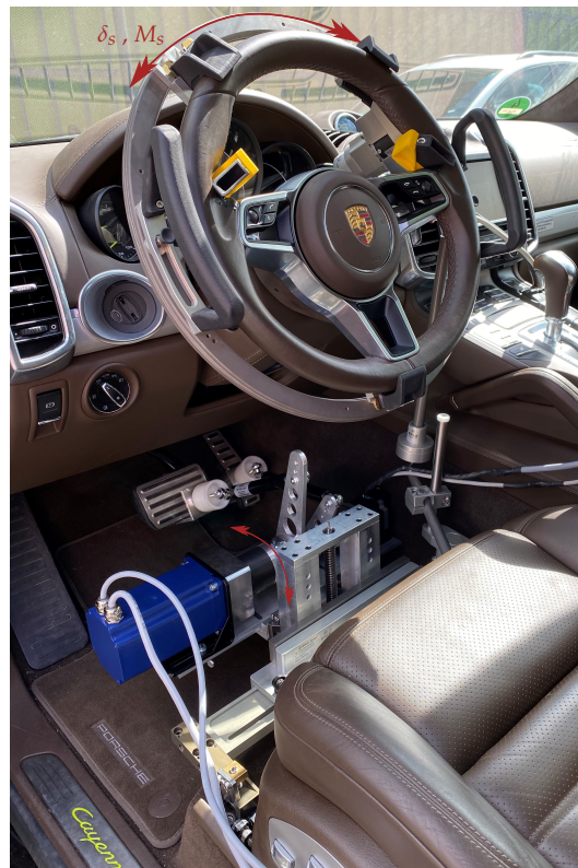
Figure 5. Driving robot consisting of a steering and pedal robot used at the test bench in a VuT.
