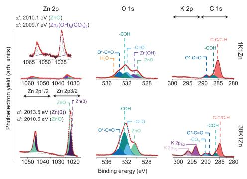
Figure 7. Zn 2p, O 1s and K 2p + C 1s photoelectron spectra of the Zn electrodes cycled in (top) 1Zn1K and (bottom) 30K1Zn electrolytes. Zn 2p inset show the calculated Zn Auger parameters.
