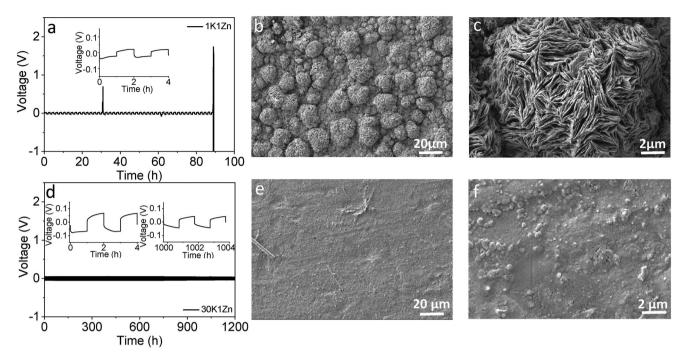
**Figure 5.** Voltage profiles recorded in a Zn||Zn symmetrical cell at 0.1 mA cm<sup>-2</sup> (each half cycle lasting for 1 h, i.e., 0.1 mAh cm<sup>-2</sup>) in a) 1K1Zn and d) 30K1Zn. SEM images of the Zn electrodes after 100 plating/stripping cycles in b,c) 1K1Zn and e,f) 30K1Zn
