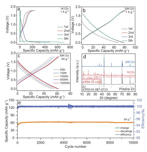
**Figure 6.** Galvanostatic charge–discharge curves recorded at Zn||AC coin cells with a) 1K1Zn and b) 30K1Zn in the voltage range 0–1.8 V at 1 A g<sup>-1</sup>. c) Selected voltage profiles and e) specific capacity and CE recorded upon galvanostatic charge–discharge cycling of a Zn||AC cell at 5 A g<sup>-1</sup> in 30K1Zn. d) XRD patterns of a pristine Zn electrode and Zn electrodes after long-term cycling in 1K1Zn and 30K1Zn.
