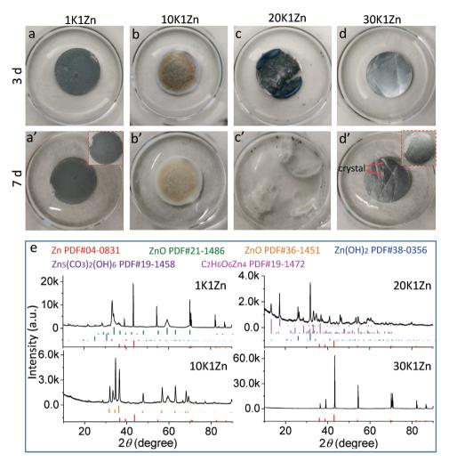
**Figure 3.** Photographs of zinc foils immersed into 0.5 mL of a,a') 1K1Zn, b,b') 10K1Zn, c,c') 20K1Zn, and d,d') 30K1Zn for 3 and 7 days, respectively. e) XRD patterns of the zinc foils (or their remainings) after a 7-day immersion into 1K1Zn, 10K1Zn, 20K1Zn, and 30K1Zn, respectively.
