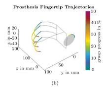
Fig. 5. Side grasp on the handle of a pitcher from the grasp database; the grasp is composed of trajectories for thumb and finger motor as well as a wrist rotation trajectory (a), the corresponding fingertip trajectories of the hand are shown in (b) together with the hand's rotation depicted as a circular trajectory.
