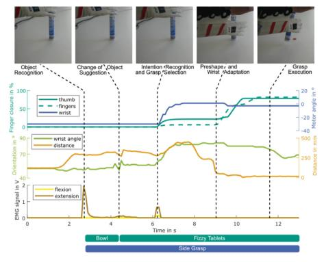
Fig. 10. Sensory data of a grasp execution with initially wrong object recognition; a clear shaking of the hand can be seen in the wrist angle measurement issued by the user to alter the object suggestion before starting the grasp.
