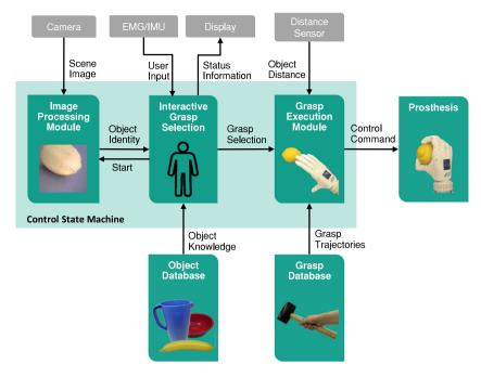
Fig. 7. Architectural diagram of the semi-autonomous control including the control state machine, sensor and feedback interfaces, knowledge databases and the prosthetic hand.
