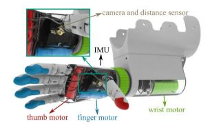
**Fig. 2.** Technical rendering of the prosthetic system with the hand and self-experience shaft; the motors actuating the fingers (blue), thumb (red) and wrist (green) as well as the distance sensor and camera (gold) are shown; the IMU is mounted on the PCB in the back of the hand.
