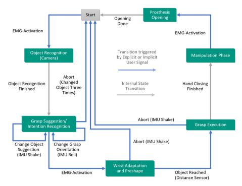
Fig. 8. Procedure of the semi-autonomous controller; throughout all grasp phases two explicit user signals are required and enhanced by implicit user input using the exteroceptive sensor information; the user can interfere at any time.
