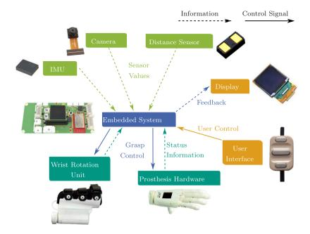
Fig. 1. Underactuated hand with two motors and ten degrees of freedom (DoF); a sensor system consisting of camera, distance sensor and IMU; a color display and an embedded system for sensor data processing and control. In addition, the wrist rotation unit and user interface, which are integrated in a self-experience shaft are shown.
