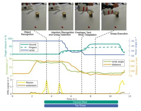
Fig. 9. Sensory data throughout one grasp execution with the semi-autonomous control; the two user inputs can be clearly seen in the EMG signal, pregrasp and grasp motion can be distinguished in the finger closure, the shaft rotation reflects the angle of the wrist throughout grasp execution and the final grasp is triggered by a low measured distance to the object.
