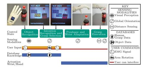
Fig. 6. Steps of the semi-autonomous controller, beginning with the first step on the left. User input is explicitly provided through an EMG signal and an arm rotation in the first two steps. Prior object knowledge in the object database is used for visual object recognition. Prior grasping knowledge in the grasp database is used for intention recognition and grasp selection. In the last two steps the grasp trajectory is performed on the prosthesis. User intervention is possible at any time.
