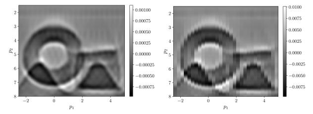
FIGURE 9. Reconstructions  $\widetilde{\Lambda}_{0.3}n$  from low resolution wave data:  $S_{\text{data}} = \Im([-10,15],101)$ ,  $\Im_{\text{data}} = \Im([17.64,47.64],7729)$ . Further,  $c(\boldsymbol{x}) = 0.1x_2 + 0.5$ ,  $\alpha = 5$ ,  $K = \Delta M^2$ , and  $\lambda = 0.1$  in (5.5). Left:  $S = \Im([-10,15],1001)$ ,  $\Im = \Im_{\text{data}}$ , and  $P_{\text{ref}} = \Im([1.5,8],86)$ . Right:  $S = S_{\text{data}}$ ,  $\Im = \Im_{\text{data}}$ , and  $P_{\text{ref}} = \Im([1.5,8],86)$ .
