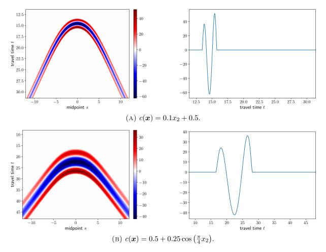
FIGURE 1. Reference kernels approximating  $v_{(0,4),0.8}$  for  $\alpha = 3$  and  $K = \Delta M^2$  with respect to linear and oscillating velocities (both velocity models are used for numerical experiments in Section 5). The cross sections on the right are taken for s = 0.
