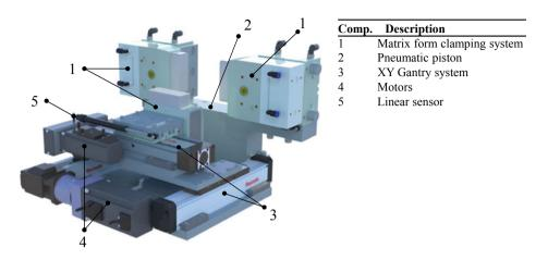
Fig. 2 CAD model of the clamping device for disassembly in remanufacturing applications
