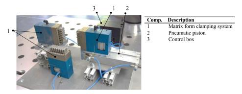
Fig. 3 Prototype system of a clamping device for disassembly in remanufacturing applications
