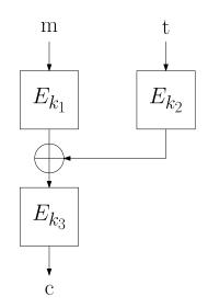
Figure 5.3.: The LRWQ Tweakable Block Cipher
