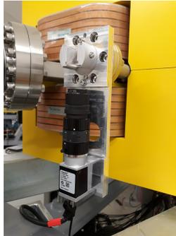
Figure 2: The experimental setup of the CCD camera in the booster.
