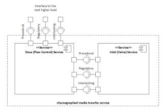
Figure 4: Schematic component model of a choreographed automation service
