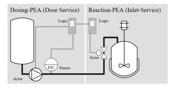
Figure 5: Technological Schema of the media transfer example
