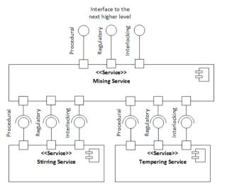
Figure 2: Schematic component model of an orchestrated automation service
