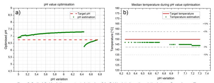
Figure 5: On the left side a), the reconstructed pH value of the fluid is plotted over its variation between five and seven. The dashed red line indicates the initial equilibrium pH at 6.743. In the right graph b), the corresponding temperature estimations are visualised, while the solid red line indicates the targeted temperature of 150°C.
