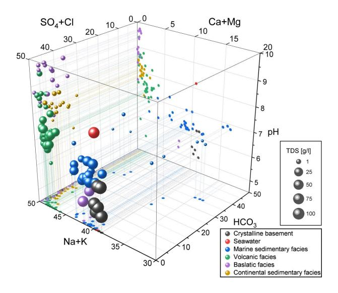
Figure 2: Modified Langelier-Ludwig diagram for classification of geothermal settings in different facies. The pH value was added as a third dimension (z-axis) as well as the total dissolved solids (TDS) visualised in sphere size.
