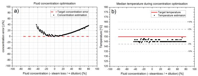
Figure 4: On the left side a), the error of the reconstructed fluid concentration is plotted over the changes to the mass of water within the fluid. The dashed red line indicates the targeted error. In the right graph b), the corresponding temperature estimations are visualised, while the solid red line indicates the targeted temperature of 150°C.
