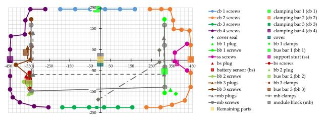
**Figure A1.** Disassembled battery system: XY–positions of the components and their connections; cb: clamping bars, mb: module block, bb: bus bar; bs: battery sensor.
