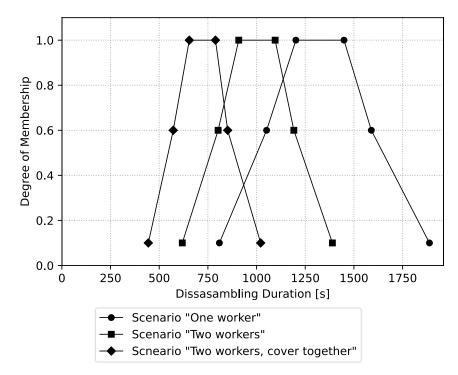
**Figure 7.** Membership function of fuzzy minimum disassembling completion time for different planning scenarios.
