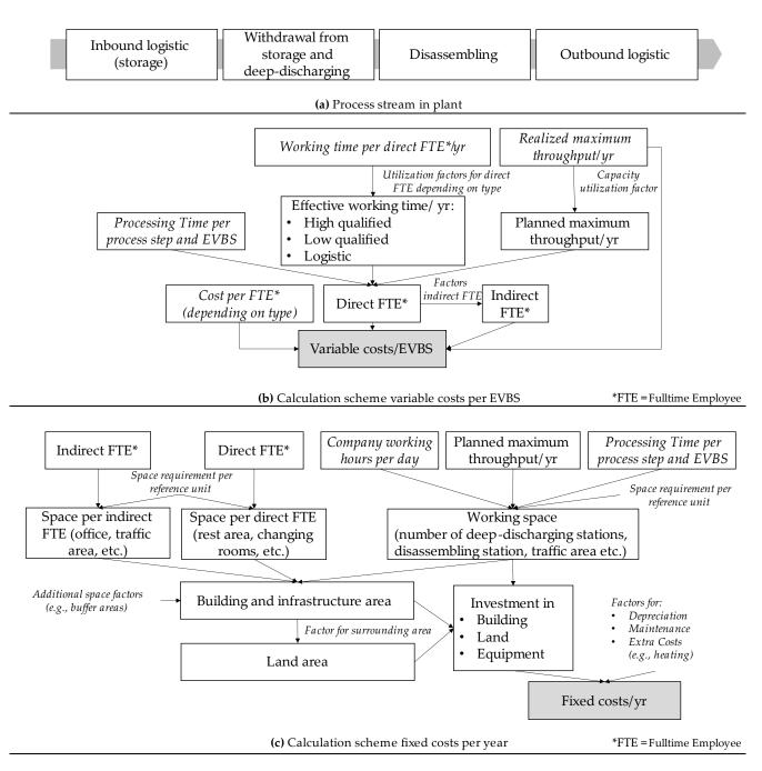
**Figure 3.** (a). Modeled process stream of the disassembly plant; (b) calculation scheme for variable disassembling costs; (c) calculation scheme annual fixed disassembling costs; explanation for (**b**,**c**) cursive text indicates that the factor is an external input for calculation.
