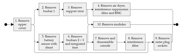
Figure 5. Disassembly graph (shortened).
