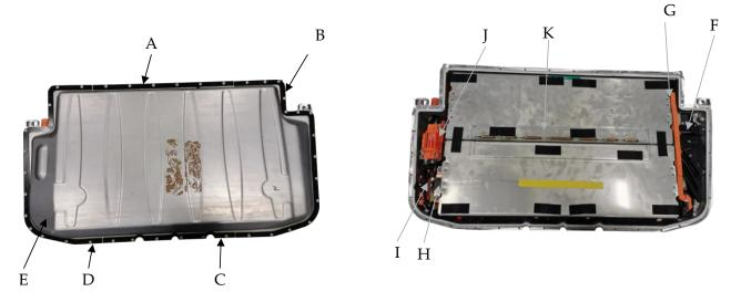
**Figure 4.** Picture of the disassembled PHEV battery system: A—clamping bar 1, B—clamping bar 2, C—clamping bar 3, D—clamping bar 4, E—cover, F—bus bar 1 (with integrated battery sensor), G—support strut, H—battery sensor (with shunt), I—bus bar 2, J—bus bar 3 (with integrated fuse), K—module block.
