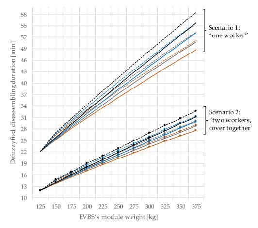
**Figure 8.** Defuzzyfied disassembling durations depending on EVBS modules' weight, workforce settings, and scaling parameters for cover removal; line colors represent different beta values for "cover removal" step: brown 0.6, grey: 0.7, blue 0.8, black 0.9; type of line represents gamma: solid:  $\gamma = 1$ ; dashed:  $\gamma = 1.05$ .
