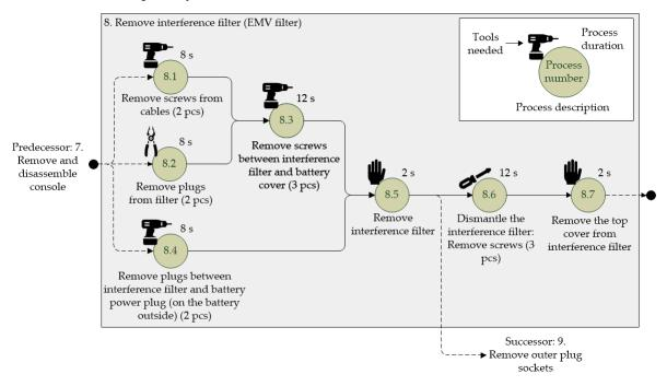
Figure 6. Detailed process description using the example "8. Remove interference filter".
