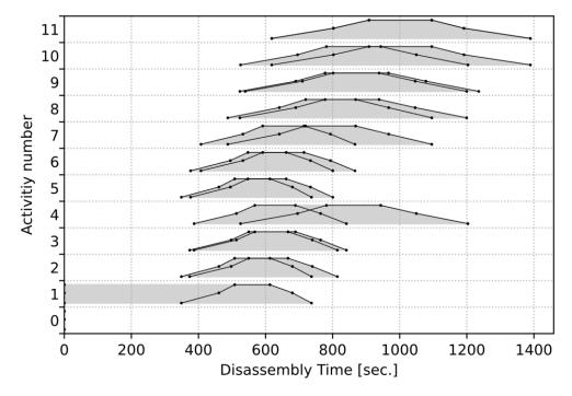
Figure A3. Scenario "Two Workers": resulting fuzzy Gantt chart for each disassembling step.
