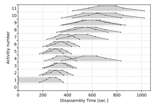
**Figure A4.** Scenario "Two Workers, cover together": resulting fuzzy Gantt chart for each disassembling step and calculated fuzzy start time  $(\tilde{t}_i^s)$  and fuzzy finish time  $(\tilde{t}_i^f)$ .
