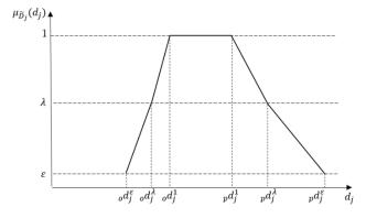
**Figure 1.** Illustrative example of a membership function based on six-point representation for a fuzzy disassembling duration  $D_i$  of process *j* (adapted from [26]).
