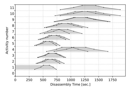
**Figure A2.** Scenario "One worker" resulting fuzzy Gantt chart for each disassembling step and calculated their fuzzy start time  $(\tilde{t}_i^s)$  and fuzzy finish time  $(\tilde{t}_i^f)$ .
