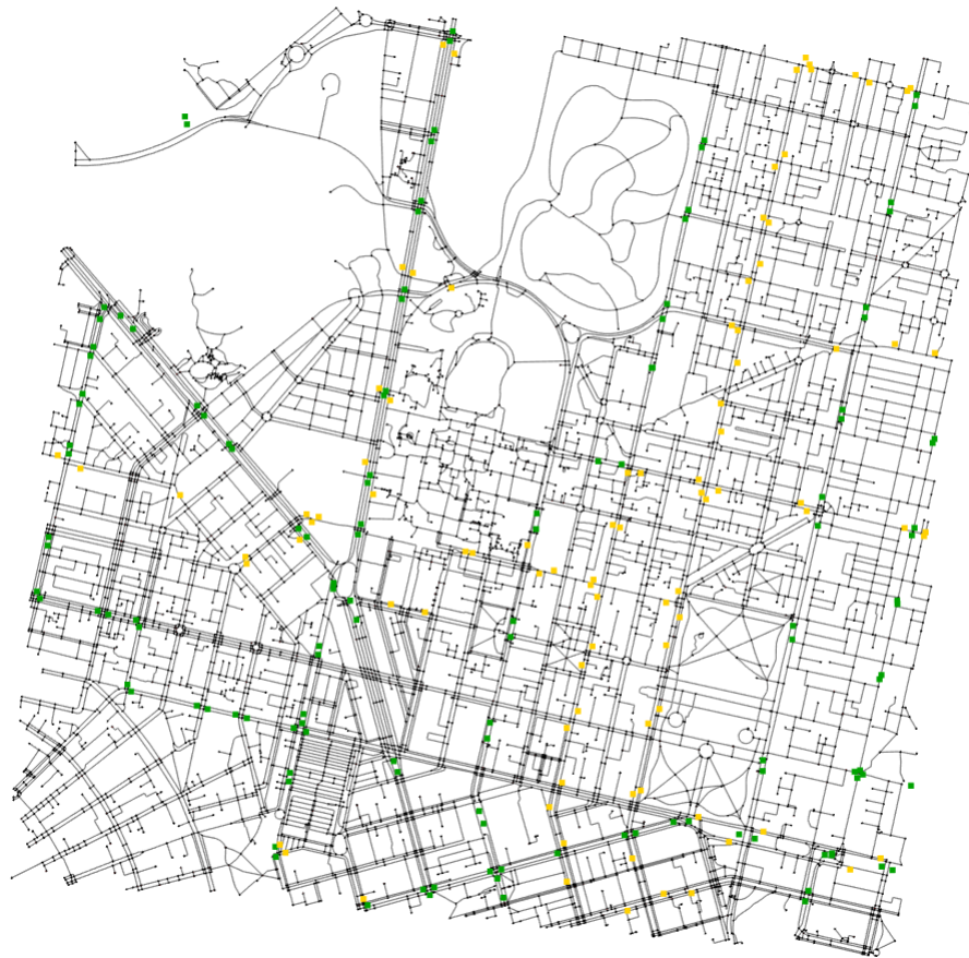
Figure 20: Pedestrian network in and around Parkville campus of University of Melbourne; green squares = tram stops, orange squares = bus stops
