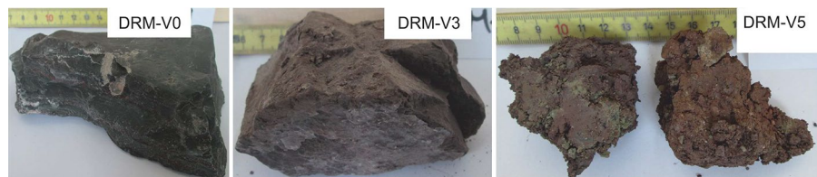
Fig. 1 Different weathered Marls from 'Dunkelroter Mergel', Grabfeld-Formation (Knopp and Moormann 2018)
