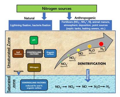
Figure 1. Conceptual model of DNT occurring in the unsaturated and saturated zones.
