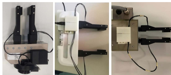
Fig. 3. Example of commercial grippers with integrated sensorized fingers: Schunk WSG-50 (left), Panda gripper (middle) and Schunk PG70 (right).
