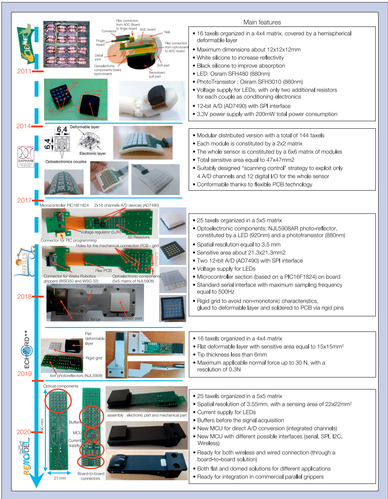
Fig. 1. Evolution of proposed tactile sensing technology. This figure uses some material, with permission, from [6] (©2012 Elsevier), [7] (©2016 IEEE), [8] (MDPI Open Access), [9] (©2018 IEEE), [10] (©2020 IEEE).
