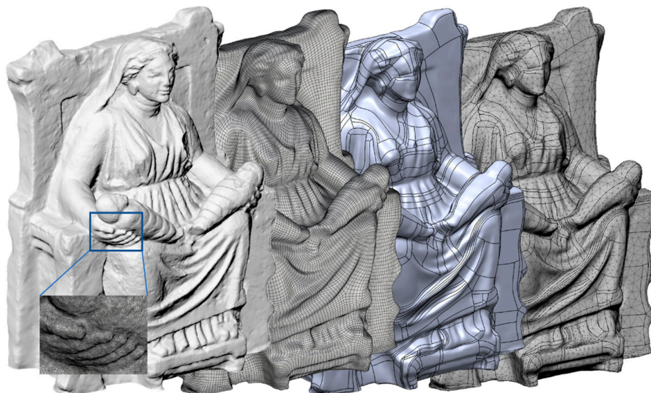
Figure 10. From the very dense scanned and tessellated model to the FE (Finite Element) mesh model, passing through the quad mesh and the surface model (from left to right).
