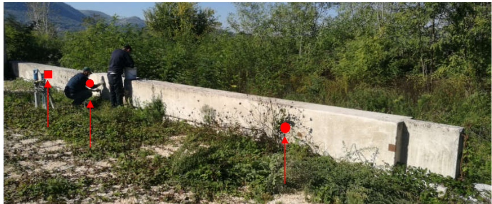
Figure 1. Precast RC squared column “C”; red circles show the location of coring sites; the red square shows the location of the extraction site of the parallelepiped-shaped diamond-cut sample.
