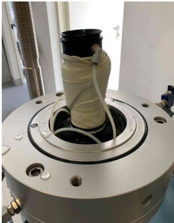
Figure 14. Failure mode of unsaturated specimens at the lowest suction value.
