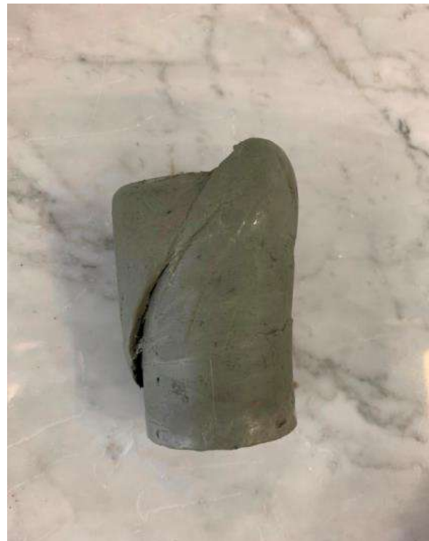
Figure 14. Failure mode of unsaturated specimens at the lowest suction value.
