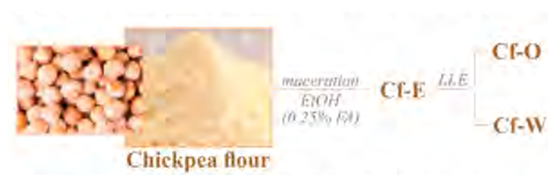
Figure 1. Extraction and fractionation scheme applied to chickpeas before UHPLC-HRMS analysis (FA = formic acid; LLE = liquid/liquid extraction).
