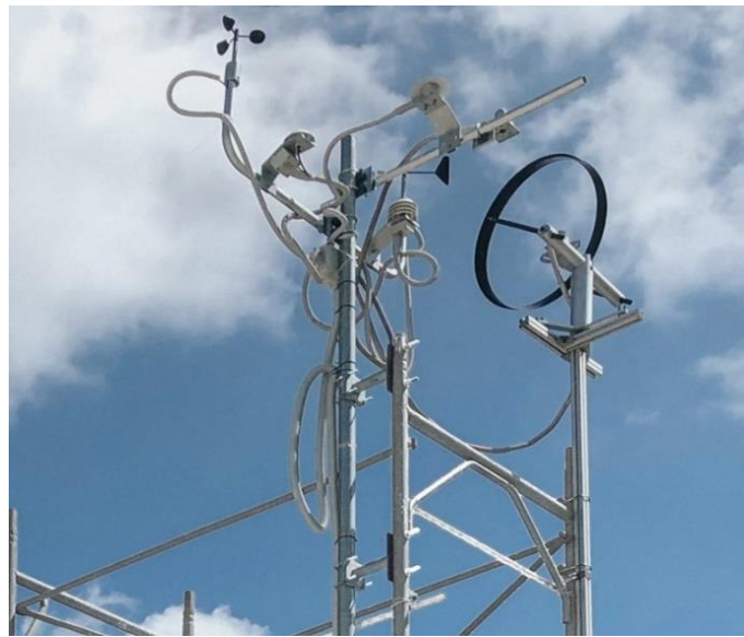
Figure 1. The weather station used to monitor the real outdoor conditions.
