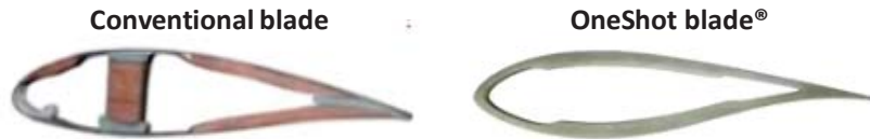
FIGURE 1. Wind turbine blade cross-section.
