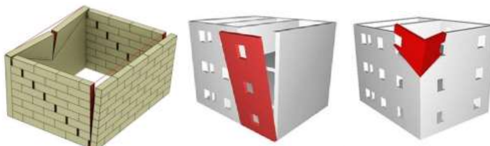
Figure 15 (a) Non-box-like behavior of the structure without decks in the event of an earthquake; (b) Simple tipping mechanism; (c). Reversal of the cantonal.
