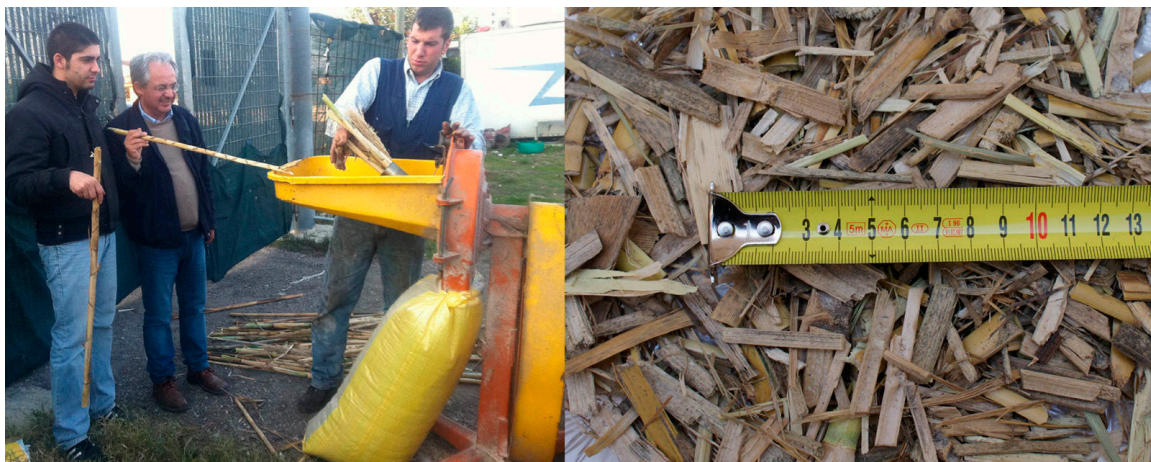
Figure 3. Detail of the shredding operations (to the left), and the average size of the crushed material (to the right).
