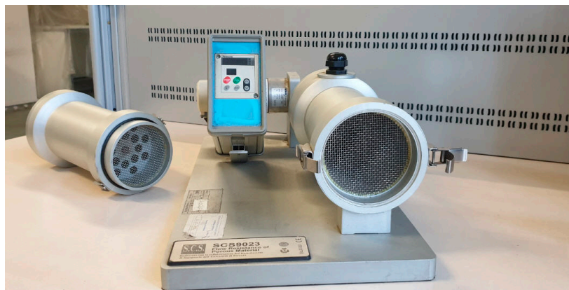
Figure 5. Air flow resistance measurements equipment with the alternating air flow method.
