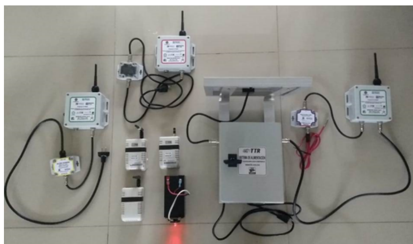
Figure 2. Wireless network with set of radio frequency nodes, coordinator node, and protective plastic coatings. Radio frequency node: country of origin: Mexico; brand: TTR; model: Node RF; \mu USB polarization: 5 V Vcc at 100 mA; polarization RJ-11 RS-485 port: 5–12 V Vcc at 100 mA; operating frequency: UHF-2.4 GHz; connection port: RS-485, USB; material: ABS plastic; dimensions: 109.5 × 70 × 38 mm; white color. Radio frequency sensor/router: country of origin: Mexico; brand: TTR; model: Node RF; RS-485 port polarization: 5–12 V Vdc at 100 mA; end devices: 100; nodes in the network: 100; jumping capacity: 15; operating frequency: UHF-2.4 GHz; connection port: RS-485; material: ABS plastic; dimensions: 120 × 120 × 60 mm; white color.
