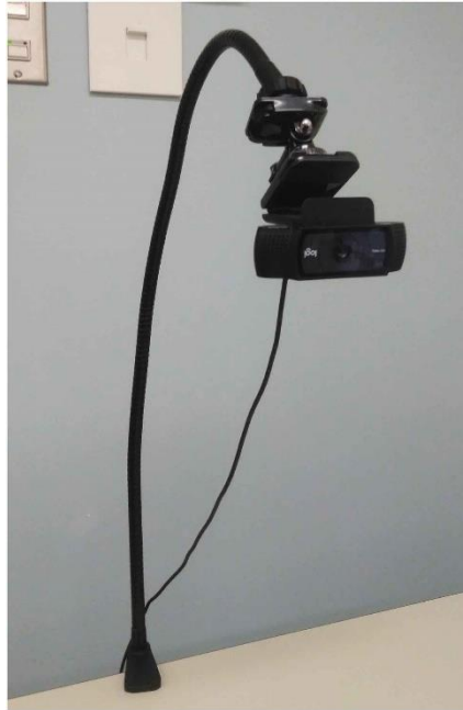
Figure 8. The gooseneck webcam mount used to lower the webcam over the edge of the monitor screen. The mount is inexpensive, easy to use, and can be locked onto the edge of a desk behind the monitor. This allows increased control over the webcam orientation and circumvents the typical limitation on downward tilting observed when the webcam is mounted directly onto the monitor.
